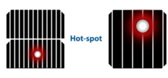
solar module. Result's show the maximum hotspot cell temperature of the shaded half-cell module is 20 °C lower than that of the full-cell module.
